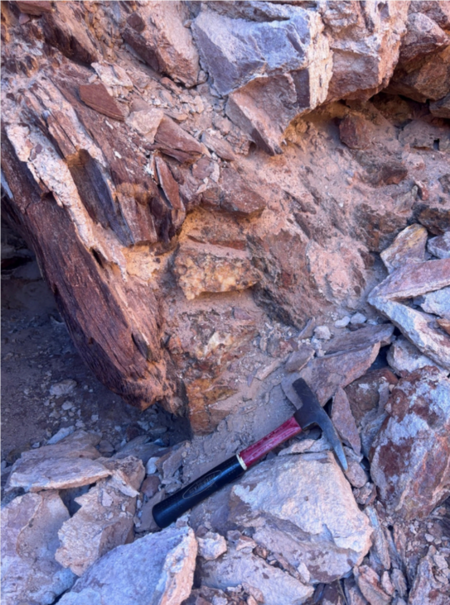
Figure 13 - 2.2 g/t qtz vein ~40cm within wall of Queen of Earth (North) workings, (GS00304)
